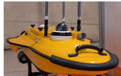
Maritime Drone with Vision System, Lithium Battery Powered
