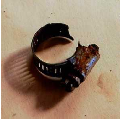
A failed hose clamp can sink your boat
